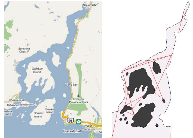
(a) Map of Howe Sound. (b) 19 patrols (guards) with unlimited range sensors cover Howe Sound. Lines show visibility between guards.
